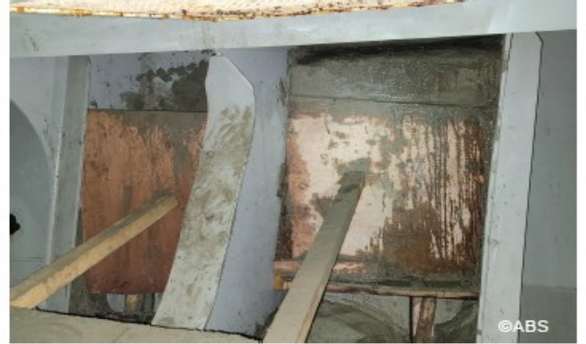
Side shell plating with cement box – temporary repair
