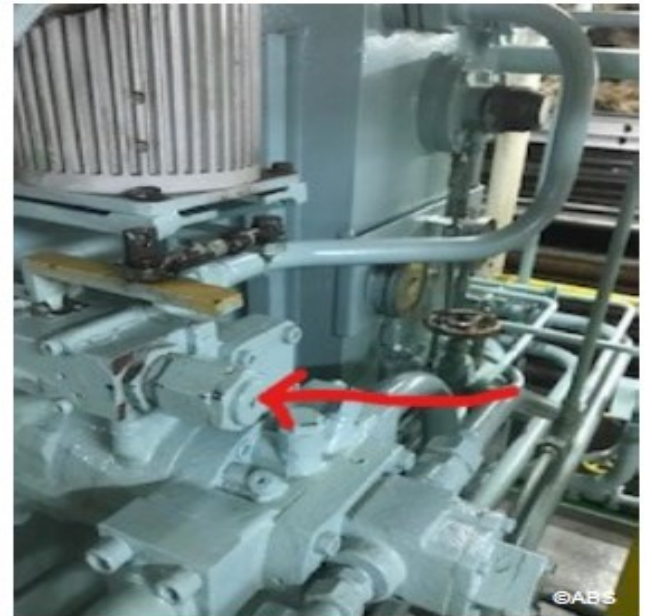
Steering gear repaired for rudder centering adjustment bolt
