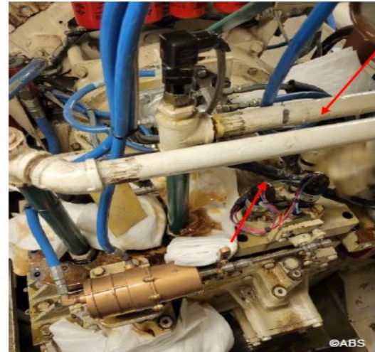
Main engine fire due to a cracked lube oil pipe fittings – before
