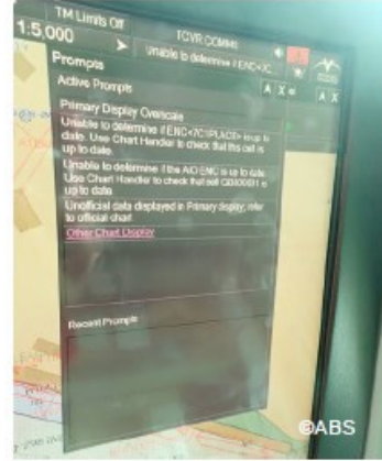
ECDIS found defective
