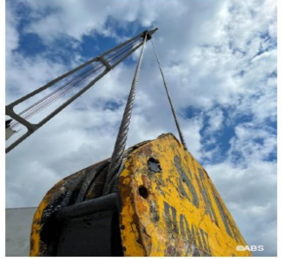
Cargo crane wire renewed – after
