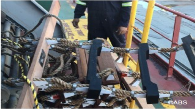
New pilot ladder provided
