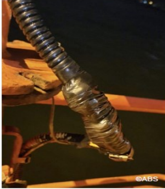
Pilot embarkation light found with electrical cables faulty
