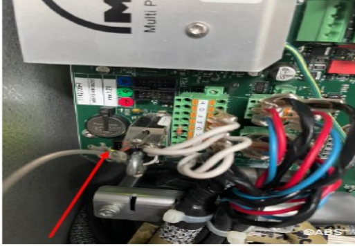
Main engine battery replaced in Engine Control Unit
