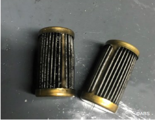
Main engine shut down due to clogged fuel injector screens
