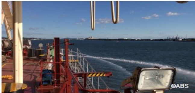
Emergency fire pump testing after repair to defective controller
