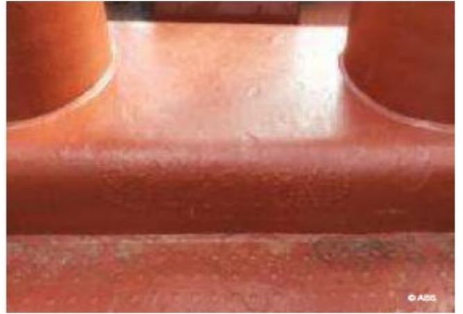
Mooring bitt not marked with SWL in contrasting color – before
