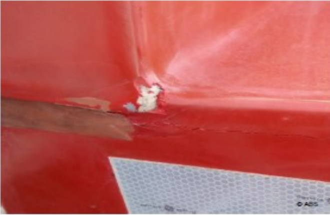
Rescue boat – hull cracks
