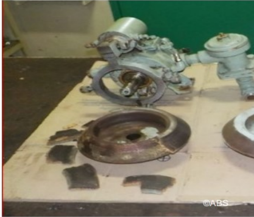
Clutch for vacuum unit of emergency fire pump broken
