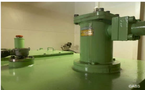
Leakage of deck machinery hydraulic pump circulating system located at Forecastle Space
